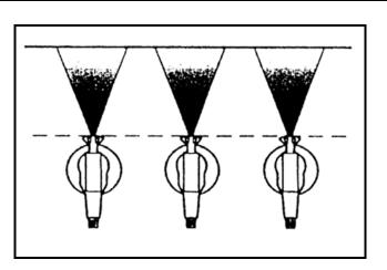
should be started before the trigger is pulled and likewise released before the stroke is ended. This gives accurate control of the gun and material.
