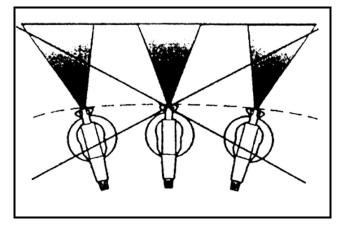
When spraying large areas, using a criss-cross pattern as shown.
